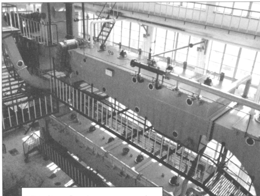
This Simon-Rosedowns extractor, designed to process 400 metric tons of sunflowerseed or rapeseed presscake per day, has been installed in Shenyang, China.
